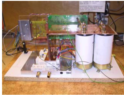
IGBT:s and the capacitors
